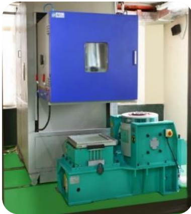
Vibration Testing Machine integrated with climate chamber
