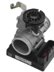
Throttle Body with integrated ECU
